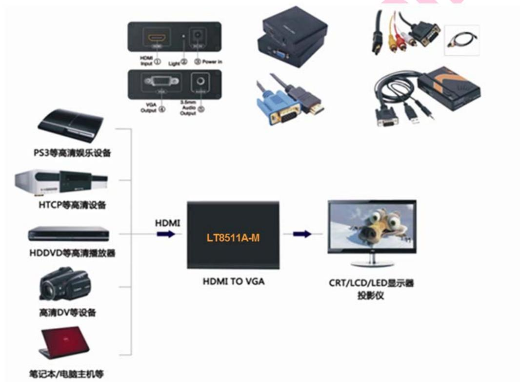
Figure 1. Application Diagram
